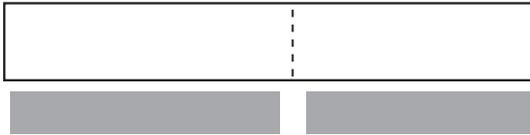
2. Cut your blank in half at that mark. **Do not cut off the extra so when drilling the blanks you have extra material to prevent a blow out and the blank being too short.**
